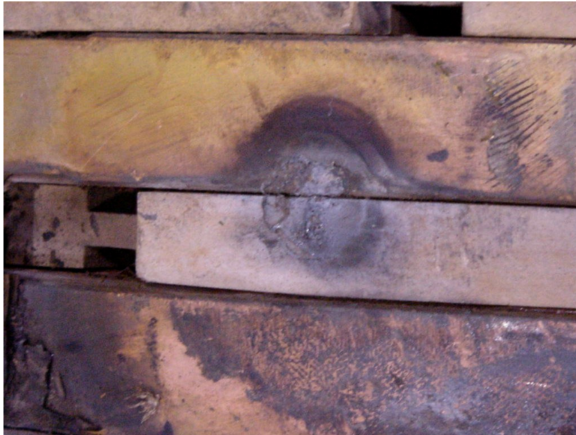
PHOTO 3 , Localized Heating at Top Turn Exciter End
