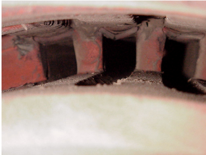
PHOTO 1 , Fractured Sub-slot Filler, Exciter End
